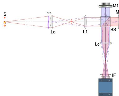
Fig. 1. (Color online) Optical schematic of IDHAO system: S, object plane, including a guide star; L, lenses; M1, piezo-mounted plane mirror; M2, curved mirror;  $\Psi$ , aberrator; IF, interference filter.
